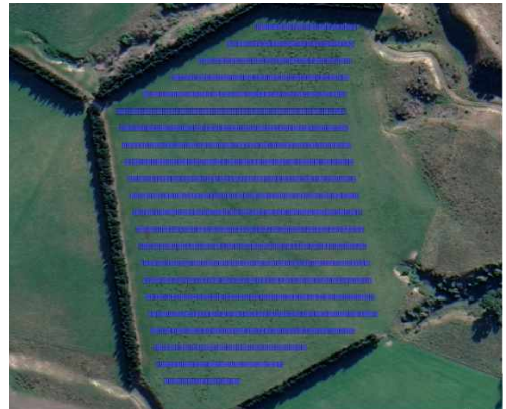
View of the fixed-tilt (top) and tracker (next page) arrangements.
